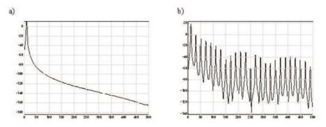
Fig. 4. Converter with dead zone: a) spectrum of input signal, b) spectrum of output signal.
