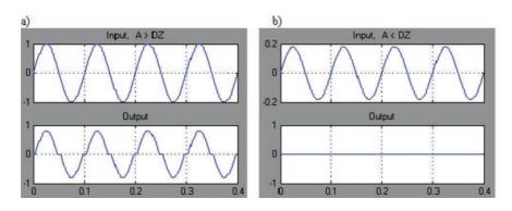
Fig. 3. Input and output signal of the converter,  $-0.2 \le DZ \le 0.2$ , a) A=1, b) A=0.18.
