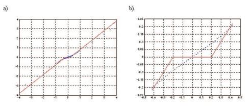
Fig. 7. Characteristic of a converter with dither: a) whole, b) fragment.
