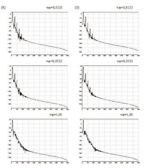
Fig. 9. Spectrum of the converter output signal,  $-0.2 \le DZ \le 0.2 A = 1$ : column (R) – dither with rectangular PDF, column (G) – dither with gaussian PDF.
