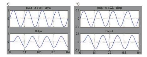
Fig. 6. Input and output signal of converter with dither  $D_{pp} = 0.4$ ,  $-0.2 \le DZ \le 0.2$ , a) A = 1, b) A = 0.18.
